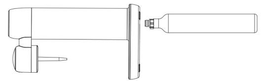
3.Load the cylinder into the machine and rotate it still firmly.
